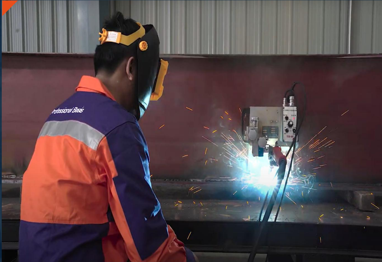
FCAW Semiautomatic Welding
